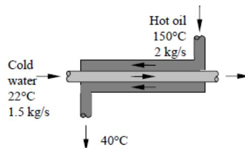
$$\begin{aligned}\dot{E}_{\text{in}} &= \dot{E}_{\text{out}} \\ \dot{m}h_1 &= \dot{Q}_{\text{out}} + \dot{m}h_2 \quad (\text{since } \Delta ke \cong \Delta pe \cong 0) \\ \dot{Q}_{\text{out}} &= \dot{m}c_p(T_1 - T_2)\end{aligned}$$
