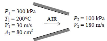
(b) We take nozzle as the system, which is a control volume since mass crosses the boundary. The energy balance for this steady-flow system can be expressed in the rate form as
