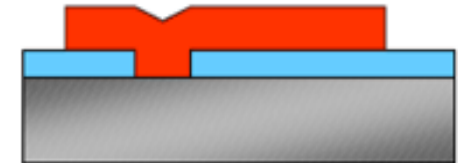
7- Structural material deposition and patterning
