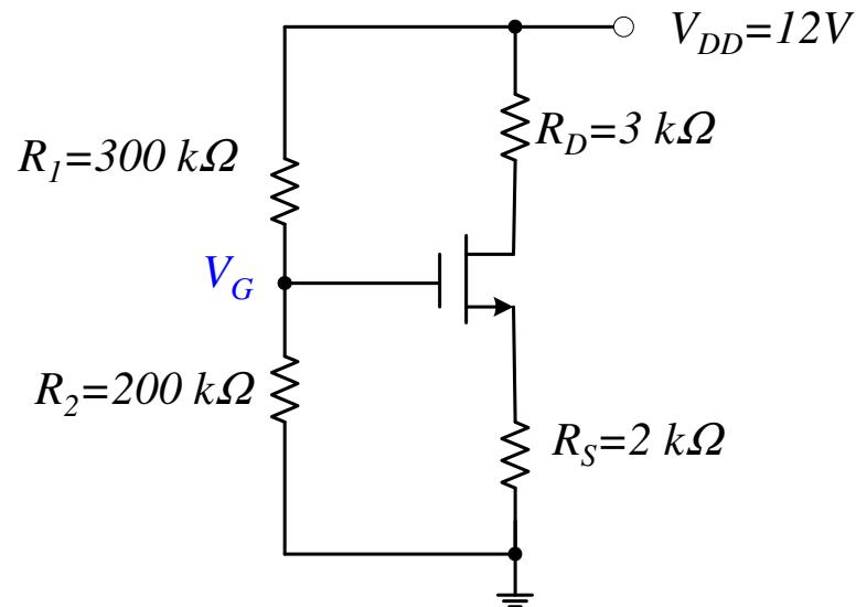
$$V_G = \left( \frac{R_2}{R_1 + R_2} \right) V_{DD} = \left( \frac{200k}{300k + 200k} \right) 12 = 4.8V$$
