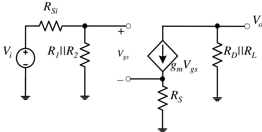
$$V_{gs} = \frac{(R_1 \| R_2)}{R_1 \| R_2 + R_{Si}} \times V_i$$
