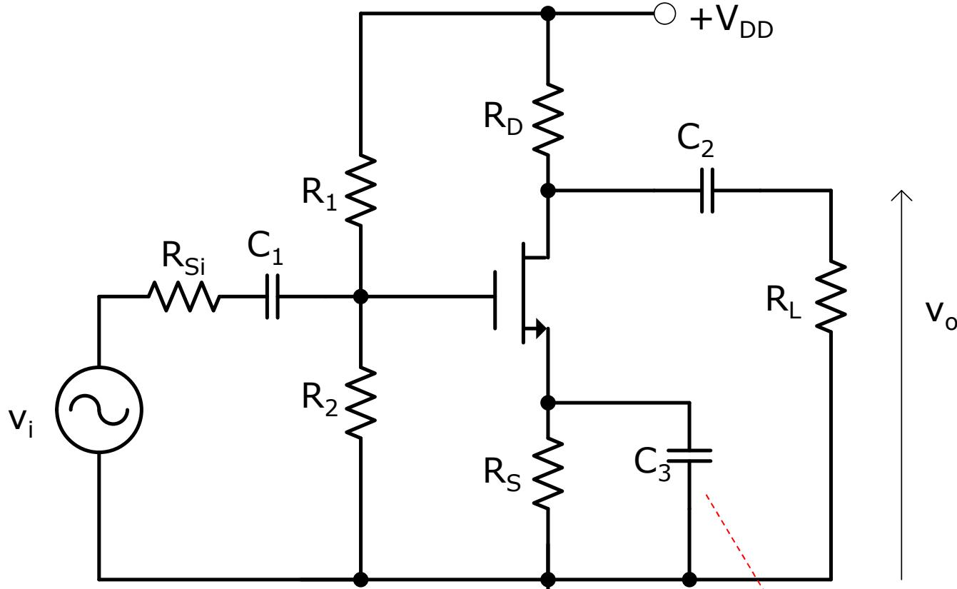
Minimize the loss in small-signal voltage gain while maintaining the Q-point stability
