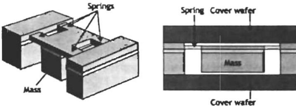
2. Design the beam suspension shown in figure. Using ANSYS as a finite element package, determine the following:
