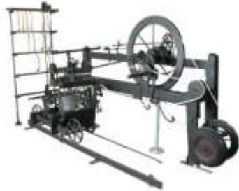
The only surviving example of a Spinning Mule built by the inventor Samuel Crompton (a combination of the Spinning Jenny and the Water Frame)
